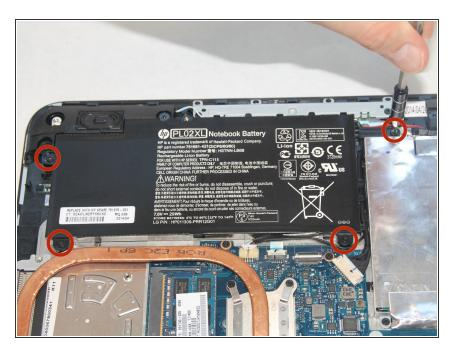
Remove the four 6mm screws from the battery with the PH0 screwdriver.
