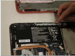
Use the spudger to pry up the blue/white speaker wires that are routed beside the battery.
