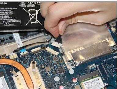
Remove the battery cable from the motherboard by gently pulling out on the black part of the cable closest to the white tab.
