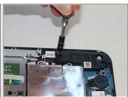
Remove two 6mm screws on each speaker with the PH0 screwdriver.
