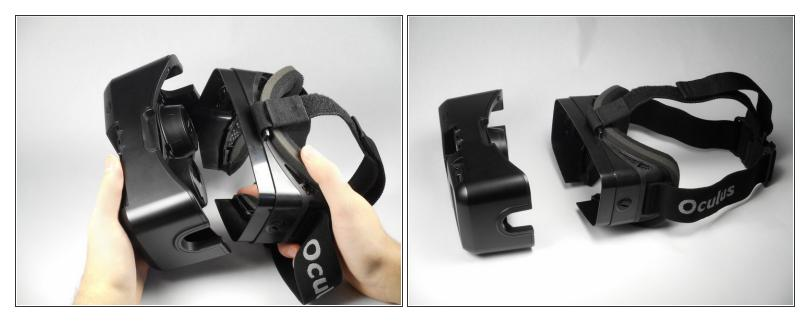
• With the screws removed, gently pull the headband frame apart from the headset.
