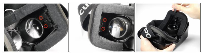
• Remove the four 3/8" Phillips #0 screws from the inner portion of the headset.
