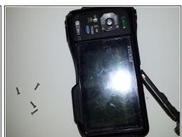
Remove the display screen from the casing. When opening, the micro USB cover and the battery cover will fall out with a pin.
