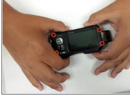
Remove 4 Phillips 1/4 inch 00 screws around the border of the display with the screwdriver.
