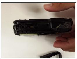
Remove the black rubber adhesive around the border of the device by peeling slowly.
