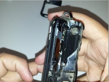
Remove 2 Phillips 00 1/4 inch rubber sealed screws off the top of the camera.
