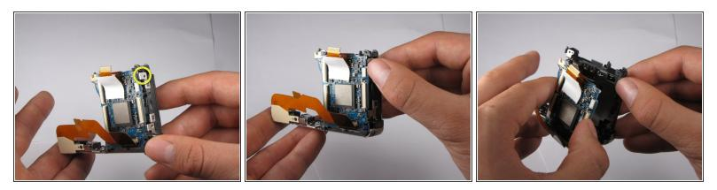
• Pull back the small gray clip located on the right side of the camera to release the motherboard from its casing.
