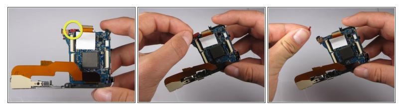
• Remove the red clip that holds the motherboard to its casing.
