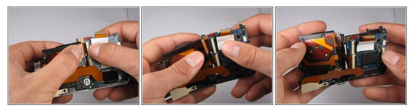
• Carefully disconnect the top ribbon-wire from the motherboard by pulling where the wire connects to the motherboard.
