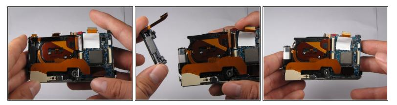
Flash capacitors are dangerous! Be *extremely* careful when removing the capacitor from the camera. You can get shocked *BADLY*!
