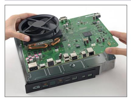
Lift the motherboard and heat sink/fan assembly out of the lower metal case.
