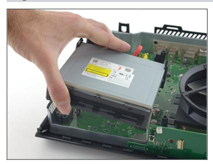
Remove the optical drive assembly from the Xbox.
