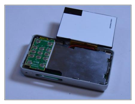
Flip the LCD screen off the midsection plate to gain access to the space around the input button chip.
