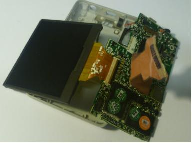
Use two fingers to peel back the edge of the ribbon connector that is glued to the bottom of the LCD screen.
