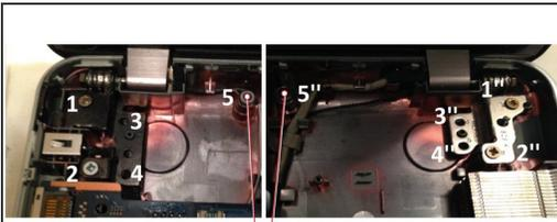
The two points are going to fix the upper part ((keyboard)) on to the base of the laptop from factory, the upper and lower art are hod together by 5 screws on left and 5 on right.
