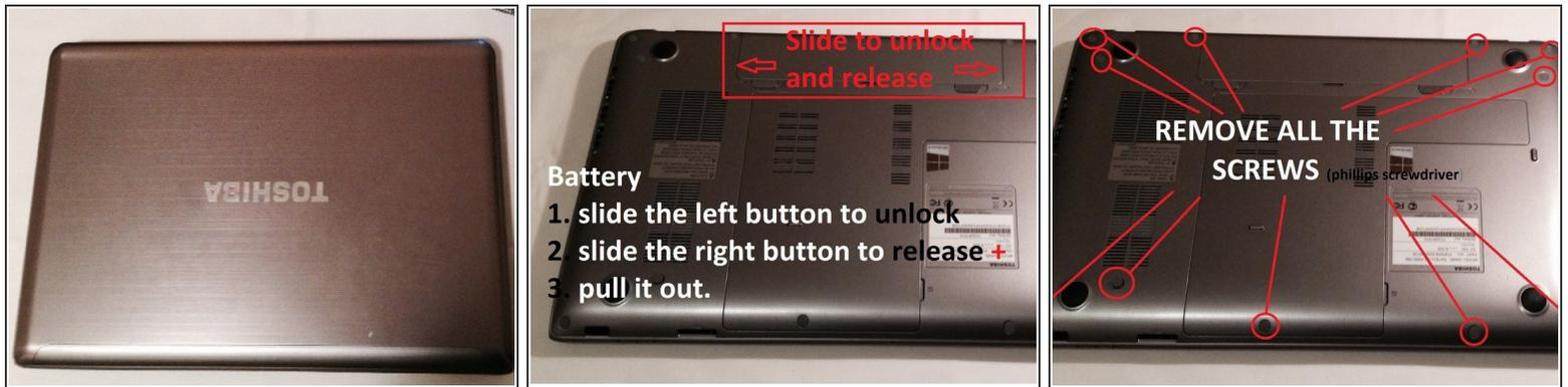
**i** To open the laptop, first you have to unscrew the back-screws.
