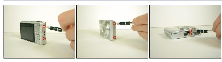
Open the battery/memory card door and remove the 6 screws (.35cm) with a Philips 000 screwdriver. There will be two screws on the left and right sides, and two on the bottom.
