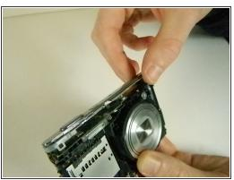
• Unscrew the .45cm screw located on the upper right corner on the back of the camera. Once the screw is off, use the spudger and unclip the piece holding the top down on the upper left on the front of the camera. It should lift off with ease.
