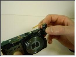
Lift the capacitor out and gently pull it away from the control board to unplug the ribbon attached to the side of the circuit board. Be careful not to bend the ribbon.
