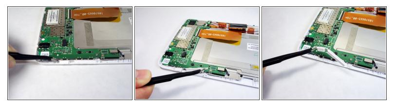
• The power button and volume buttons are together as a single piece. Gently pull up on one side and then pull up on the other side to remove the buttons from the casing.
