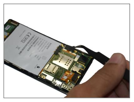
Then remove the sticky pad located at the left of the phone using he tweezers.
