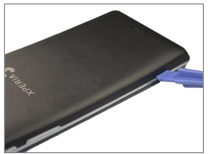
• Find the little bracket on the bottom left of the phone (when looking at it upside down) and use the opening tool to pry off the back cover.
