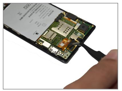
Using the <u>tweezers</u> remove the clip located at the top of the phone. It should snap right off without too much pressure.
