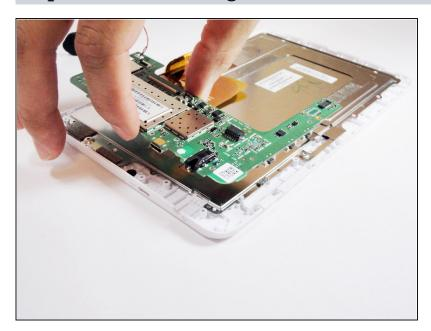
Carefully lift the motherboard directly up.
