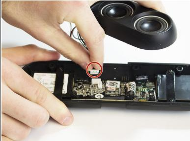
Carefully remove the control cables (4 black, 1 red).
