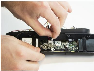
Carefully remove the black and red NFC sensor wires.
