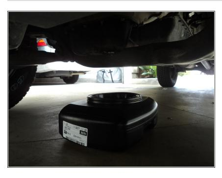
Place the drain pan under the drain plug so it will catch the oil as it falls vertically from the engine.
