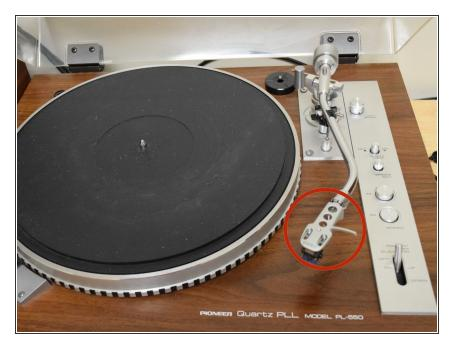
Identify the headshell by opening the turntable dust cover.
