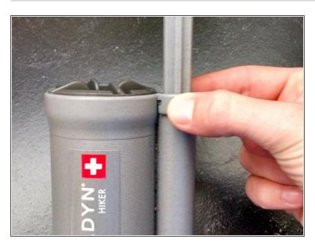
Remove the "snap fit" guard by pulling directly away from the filter body.
