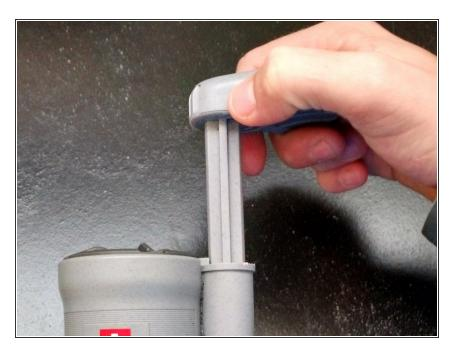
Remove the pump handle by pulling it completely out of the shaft.
