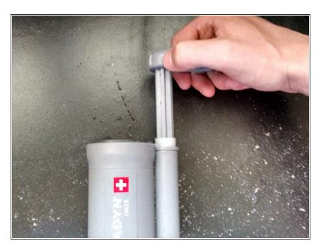
Replace the pump handle inside the pump handle shaft.
