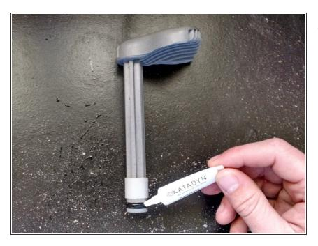
Lubricate the pump handle O-ring extensively with the Katadyne lubricant (sold with pump).
