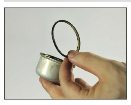
Inspect the O-ring inside the carburetor tank. If it is dry and worn out, you may need to replace the Oring before you reassemble your device.
