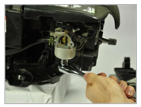
Use a socket wrench with a ½" hex bit to remove 11mm screw on the bottom of the tank.
