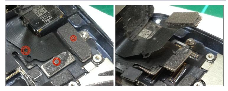
• Locate **three cables** that link from the back of the display assembly to the logic board.
