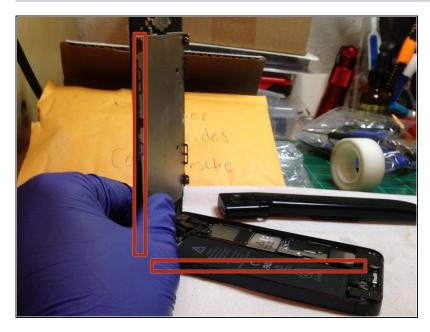
Gently lift the display assembly away from the phone, and make a 90 degree angle with respect to the horizontal.
