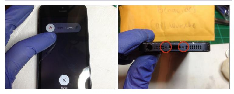
$\triangle$  Before removing the Display assembly, be sure to power off your phone. This can prevent power shortages.
