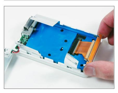
Slide the hard drive cable out of its connector.
