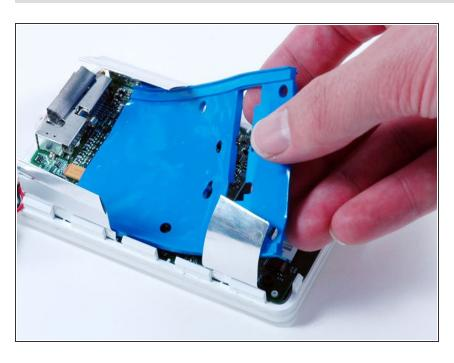
Lift the blue hard drive mounting bracket out of the iPod.
