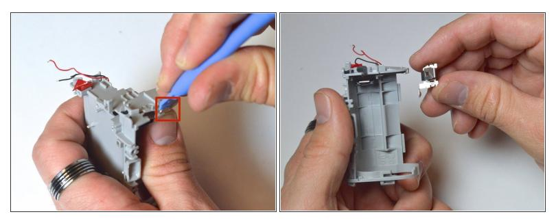
Use the plastic opening tool to unclip the metal tab.
