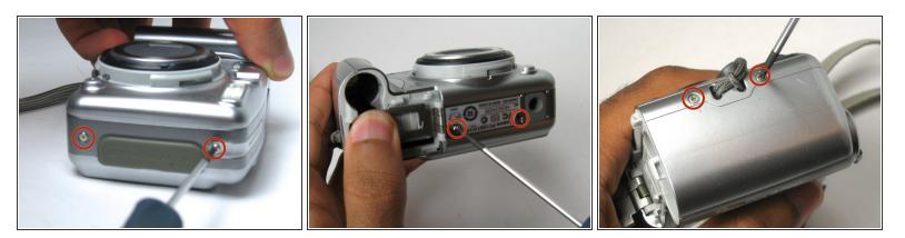
• Remove the six 4 mm Phillips head screws on both the sides and bottom of the camera.
