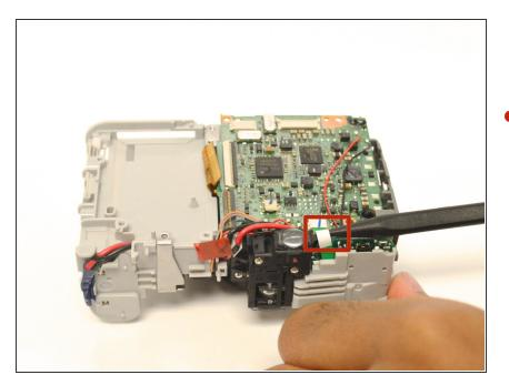
Use the spudger to remove the green ribbon from the attached ZIF connector.
