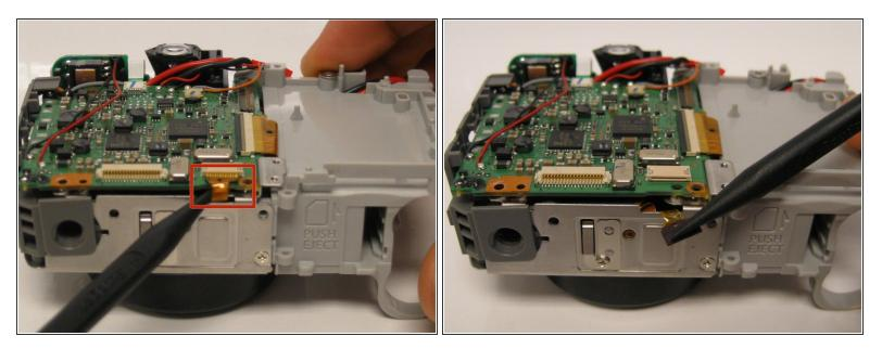
Use the spudger to remove the attached ribbon cable. Be sure to alternate the spudger on both sides of ribbon cable to remove evenly.
