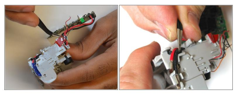
• Use tweezers to remove the tape and rubber strap. Unravel the wires from the plastic hooks.
