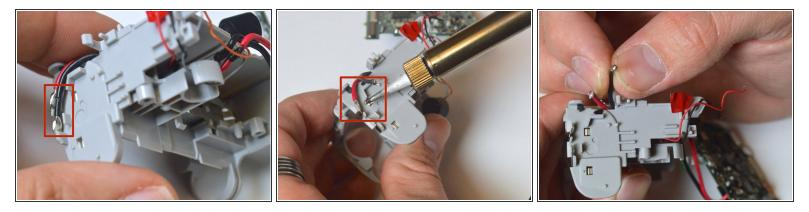
• Use the soldering iron to remove the red and black wires from the battery contacts.
