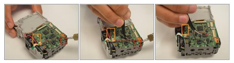
• Desolder all of the wires attached to the motherboard and move them aside with the tweezers.
