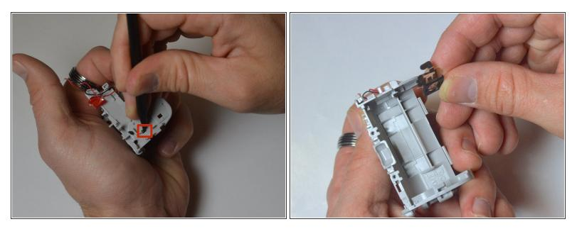
Apply pressure with the spudger to detach the clip.
