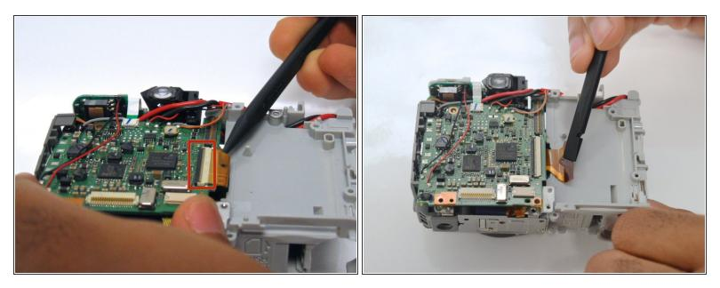
• Use the spudger to remove the pictured ribbon from the ZIF connector.
