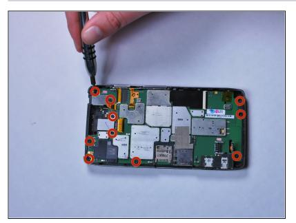
Unscrew all ten 4.0 mm screws on the motherboard using a T5 Torx screwdriver.
