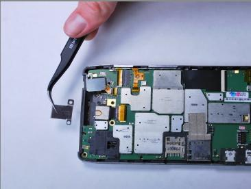
• Using tweezers, remove the back facing camera cover.
