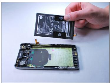
• Wedge the spudger tool under the battery to remove it from the back case.
