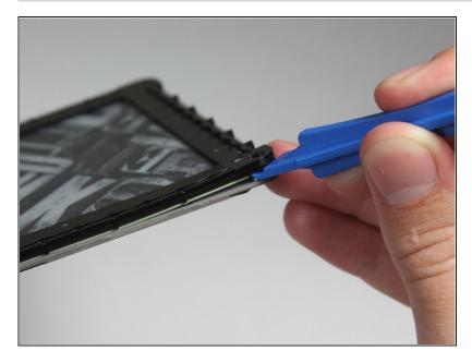
• Run the plastic opening tool around the edge to separate the bezel from the adhesive.
