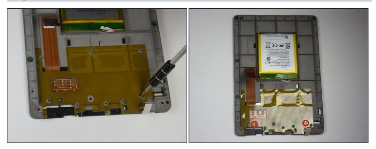
• Remove the two 2.5 mm Phillips Head screws using the T5 Torx screwdriver.
