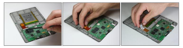
• Use the tip of the spudger to flip up the small retaining flap on the copper colored zero insertion force (ZIF) connector.
