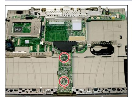
• Remove the two long silver Torx screws from the power card in the center of the laptop
