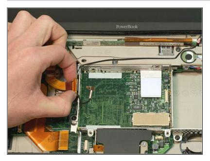
Grasp the orange display data cable and disconnect it from the logic board.
