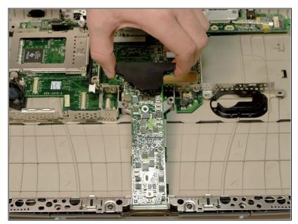
• Grasp the power card near the black shield and lift up.
