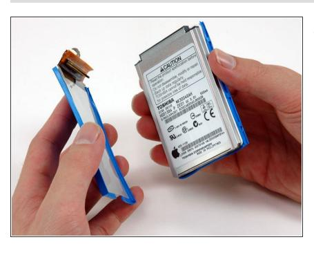
Lift the hard drive mounting bracket and cable off the hard drive.
