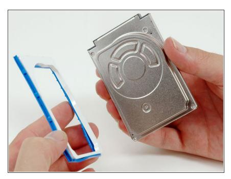
Lift the blue and white mounting bracket off the other side of the hard drive.
