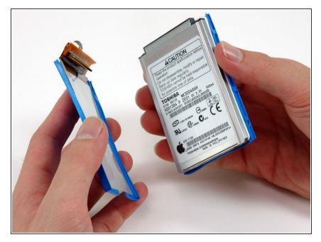
• Lift the hard drive mounting bracket and cable off the hard drive.
