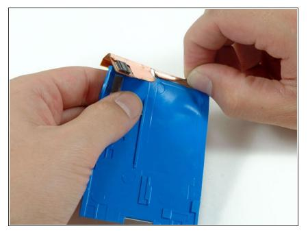
Peel up the metallic tape holding the hard drive ribbon to the blue mounting bracket.
