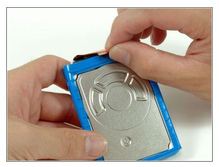
Peel back the metallic tape connecting the hard drive ribbon to the blue mounting bracket.
