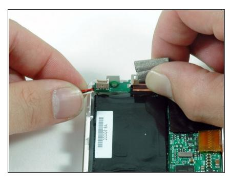
Carefully thread the battery cable around the end of the logic board.
