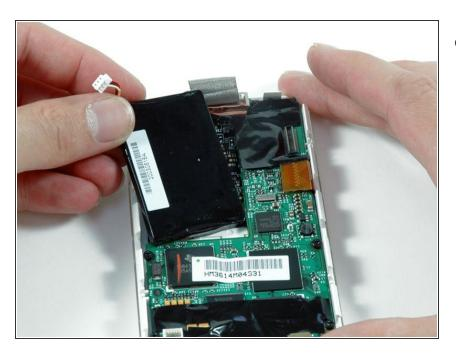
Lift the battery up and out of the iPod.
