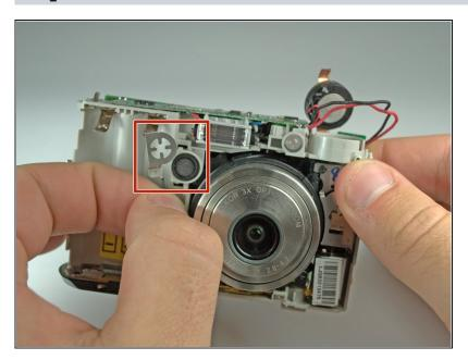
Remove the cross-hair shaped wire cap to the left of the lens.
