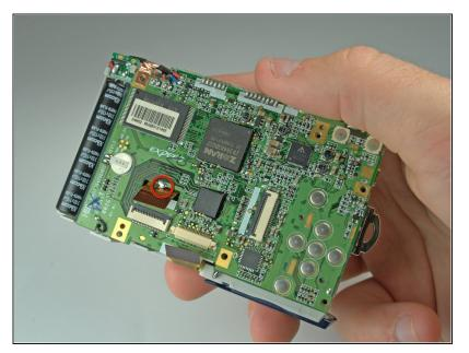
Desolder the connection of the motherboard to the lens ribbon using a soldering iron and desoldering wick.
