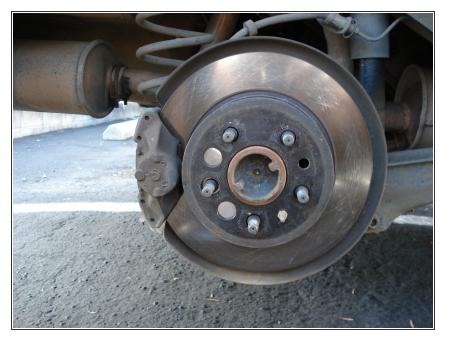
Remove tires by pulling directly away from car exposing brake rotors.
