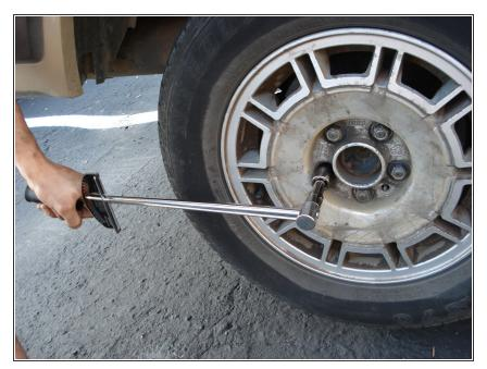
• Loosen each of the five lug nuts on all tires by turning them counterclockwise with a 19mm wrench.
