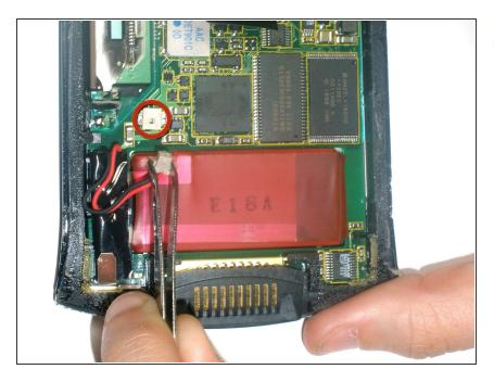
Using the tweezers, carefully disconnect the battery cable from the port
