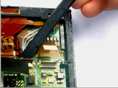
Using the spudger lift the tabs holding the LCD/Digitizer combo cables to the WorkPad.
