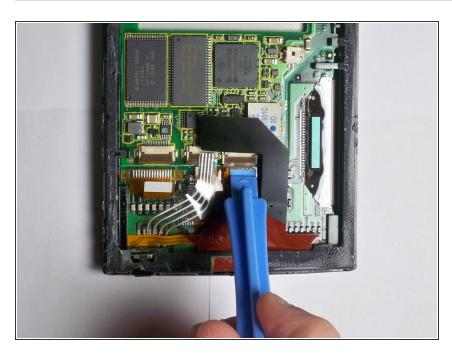
Using the plastic opening tool, lift the clip holding the motherboard cable.
