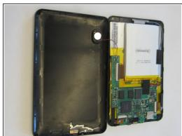
Remove back cover with lever tool, exposing the battery and motherboard.
