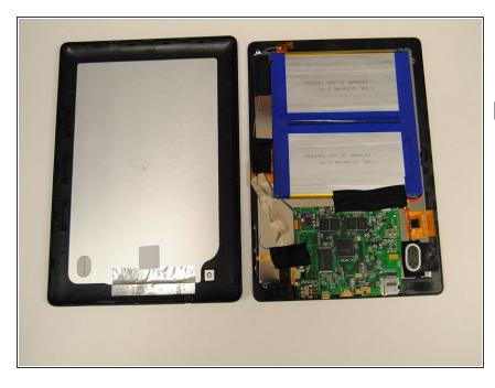
• Remove the back cover of the tablet to reveal the internals.
