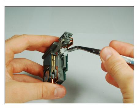
Use tweezers to remove the small white piece from the motherboard assembly.
