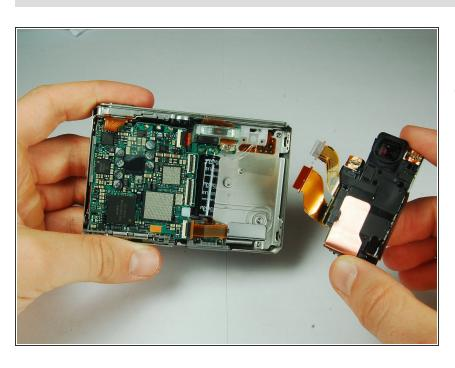
Grasp the CCD Sensor Module and remove it. To reassemble your device, follow these instructions in reverse order.
