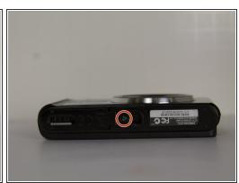
Use a Phillips head screwdriver to remove 5 screws from the camera. There are 2 4mm screws on the left side, 2 2mm screws on the right side and 1 4mm screw on the bottom.
