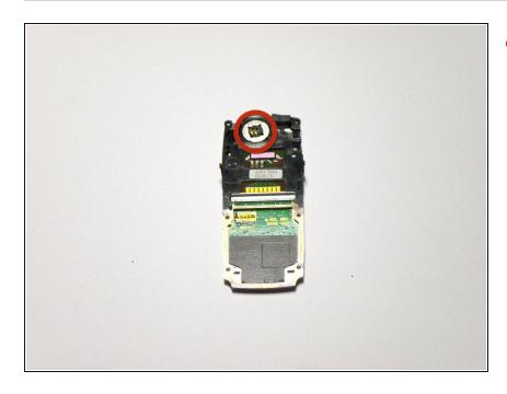
• Locate speaker on the back of the assembly.
