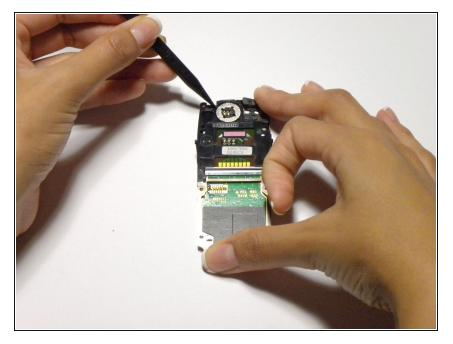
• Insert spudger under upper left side of speaker and gently lift to remove
