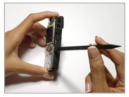
Insert spudger along edge of assembly and gently lift assembly away from case
