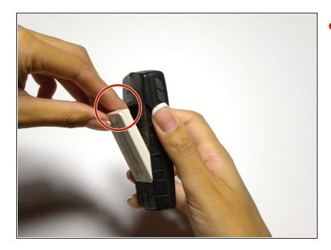
• To remove the battery, push it down from the top and pull it out.
