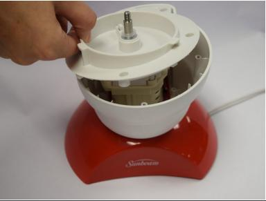
Unscrew the five screws and remove the piece labeled in the picture. You should now be able to see the motor.
