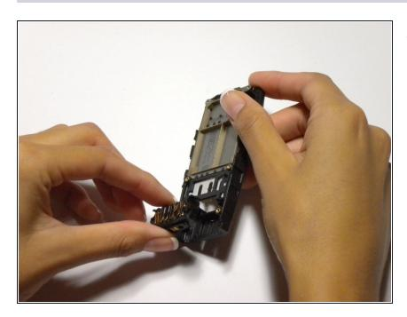
Lift out the battery charger connector
