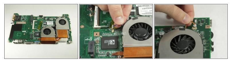
• Remove cables connecting the fans with the motherboard.
