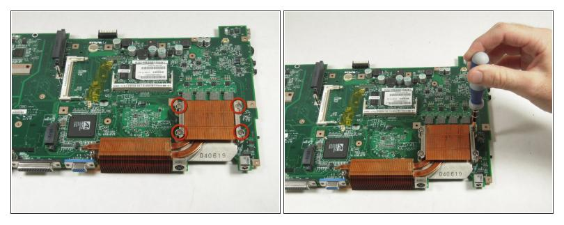
• With the phillips screwdriver remove the four screws holding the heatsink on the motherboard.
