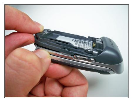
Using your fingernail lift up the side of the casing around the bottom of the phone to release all five of the clips.
