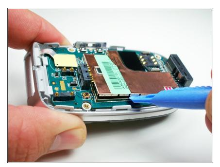
Use a plastic opening tool to lift up the brass colored panel.
