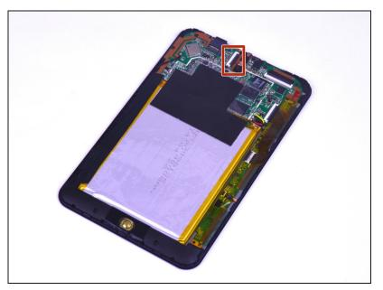
Use your fingers to pull the latch upwards to unlock the ribbon cable.
