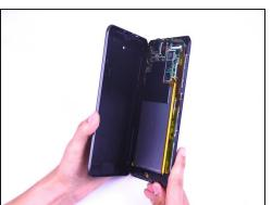
• Use an opening tool to pry open a corner of the device, then slide the tool down the side of the device to completely open it.
