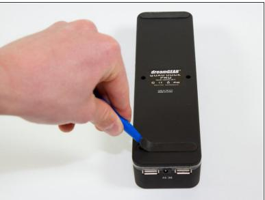
Remove the rubber foot pads on the bottom of the device using a plastic opening tool.
