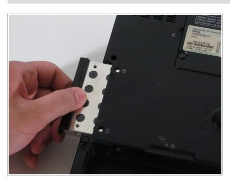
Slide the hard drive tray out of the hard drive compartment. To reassemble your device, follow these instructions in reverse order.
