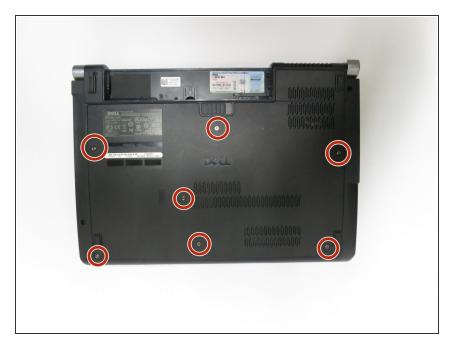
Unscrew and remove all of the 6.0mm screws with a Phillips #1 screwdriver.
