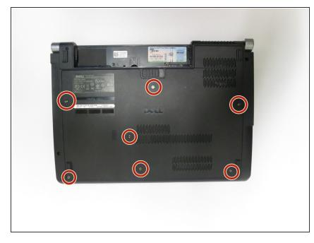
Unscrew and remove all of the 6.0mm screws with a Phillips #1 screwdriver.
