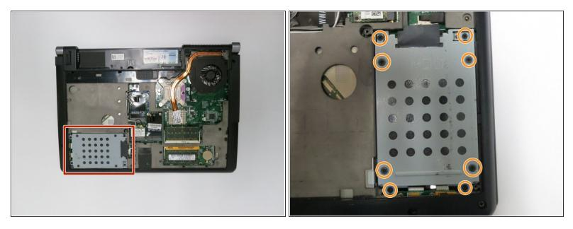
Unscrew all of the 6.0 mm screws with a Phillips #1 screwdriver holding the hard drive cage on the computer.
