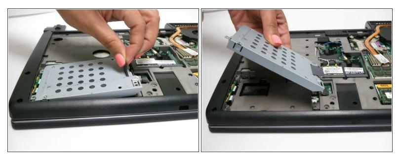
• Lift the hard drive cage out of the laptop.
