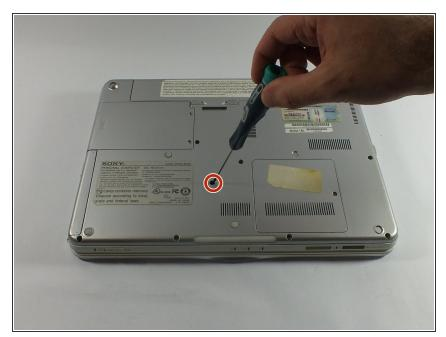
Using a #00 Phillips screwdriver, remove the screw
