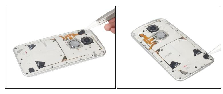
Remove those two rubber covers which securing power button connecting flex connector and battery connector.
