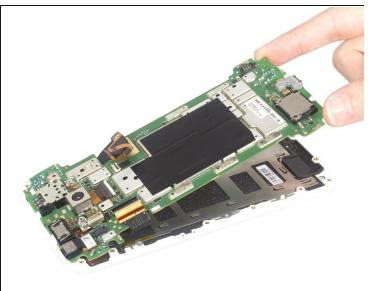
Pry up the motherboard from right and bottom corner. Remove the LCD screen from motherboard.
