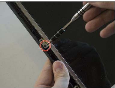
Remove the two 6mm Phillips #0 screws on either side of the screen using a Phillips #0 screwdriver.
