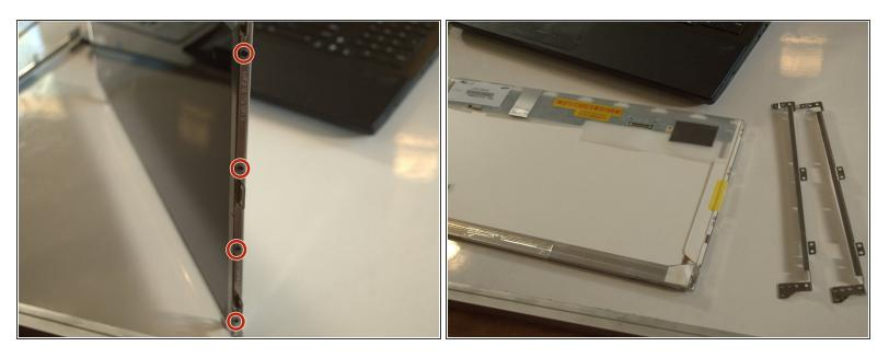
The last step is to remove eight 3mm Phillip #0 screws from both side brackets of the screen itself using a Phillips #0 screwdriver. There are four screws on each side.
