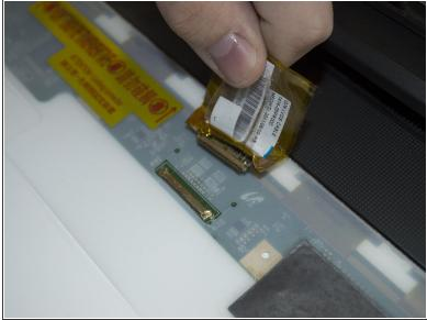
Remove the screen from the laptop casing and flip it over. Peel the sticker above the connector back and firmly pull the connector out.
