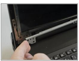
Repeat the last step with the bottom bracket, removing eight 6 mm Phillips #0 screws using a Phillips #0 screwdriver. Set the bracket aside.
