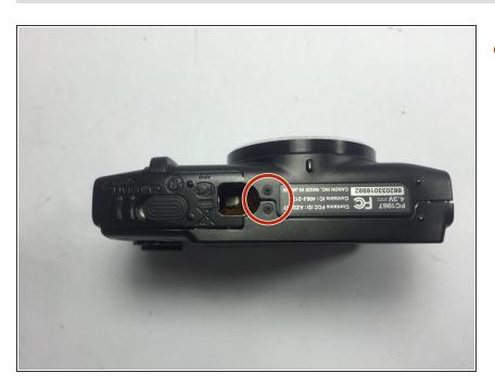
Finally, there are two screws on the bottom that need to be removed, which are marked in the photo.
