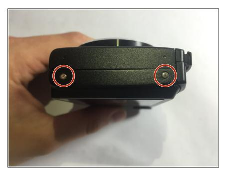
There are two screws in the left side of the camera, which are marked in the photo. Remove these screws first.
