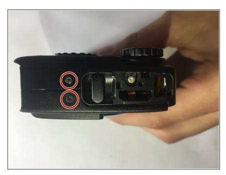
There are two screws to remove on the right side of the camera as well, as marked in the photo. Remove these screws next.
