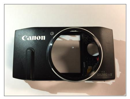
Now you can place a new camera case on the camera. As said in the step above, be wary of leaving the case off for too long, as this could damage key components in the camera.
