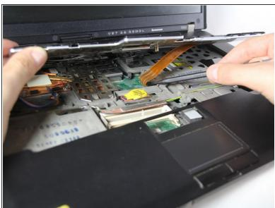
While lifting the panel, lift the keyboard up.
