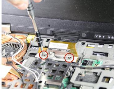
Remove the two 3mm screws next to the lid hinges, as well as the two 3mm screws on the lid's ribbon cable.
