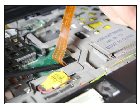
• Disconnect the ribbon cable with the spudger.
