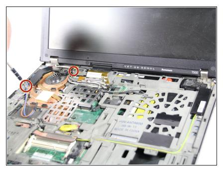
Remove the two 3mm screws on the left speaker with the Phillips #0 Screwdriver.
