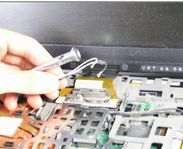
• Using the Phillips #0 Screwdriver, lift the metal fastener up and remove the black and white wires.
